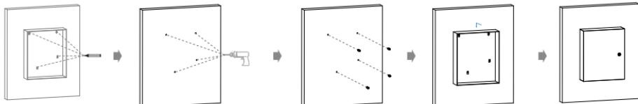
Place the EC32 in the position where it needs to be installed and mark four holes of the back cover on the wall.
